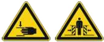
**Warning! Danger of bruising during transport and unpacking of the pv panels!**
